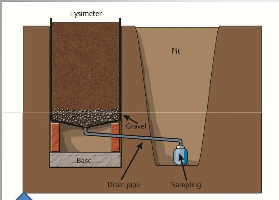
↑ Underground deployed field lysimeter
