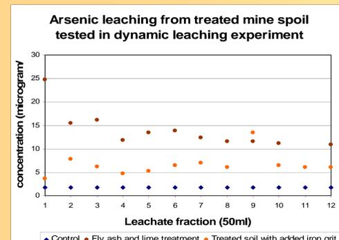
Chart 3: Leachable metal content drops in field experimental plots treated with 5% fly ash, 2% slack lime, and 0,5% iron grit, dynamic leaching test
