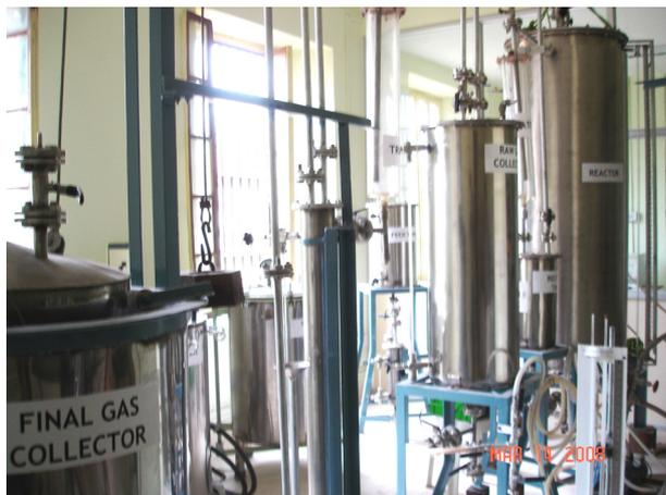
Fig. 1. Pilot plant studies ( $800 \text{ dm}^3$ ) at Indian Institute of Technology Kharagpur, India, using immobilized *Enterobacter cloacae* IIT-BT 08 for hydrogen production from cane molasses.
